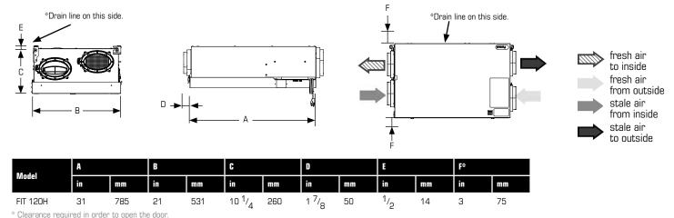
Clearance of 8" (203 mm) on the bottom of the unit is recommended for removal of core. All units feature three foot plug-in power cord with 3-prong plug.
